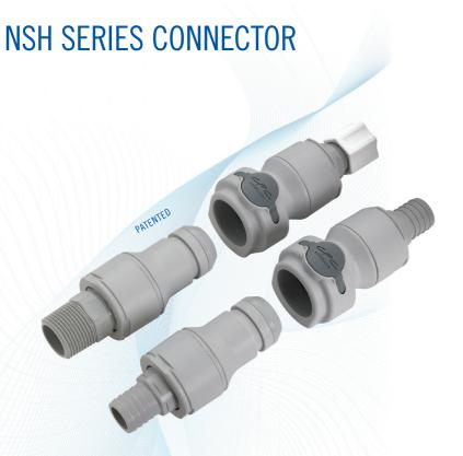
NSH Series couplings couplings are general purpose versions of our pressure-balanced, non-spill, ChemQuik® CQG06 couplings. Molded polypropylene, EPDM seals and a 100% springless and metal-free flow path provide broad chemical resistance and exceptionally high flow capacity, allowing instant disconnects (and reconnects), even under pressure. Their non-spill design virtually eliminates spills, minimizes downtime and enhances operator safety in a very low cost package.
