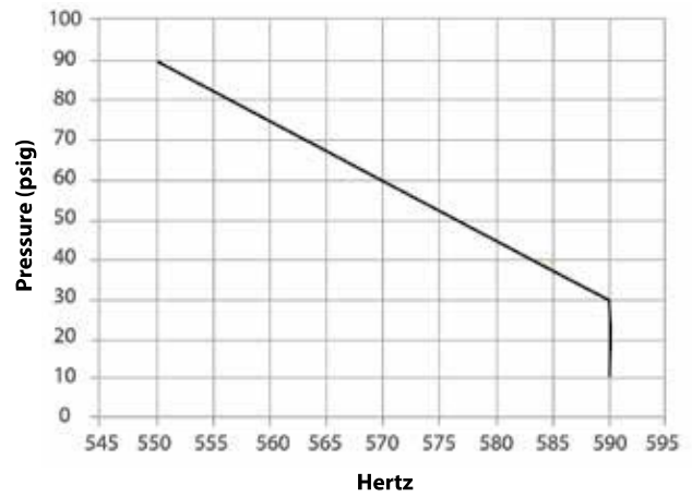
Maximum Step Pulse Frequency vs. Operating Pressure
