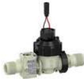
52.007.126 DN 7; 0,5 - 10 bar; 18 l/min @ 1 bar
