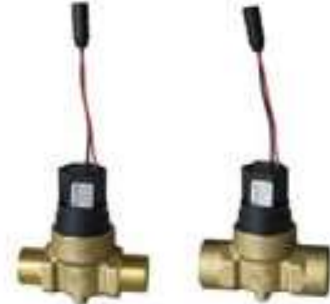
50.007.52x (Brass) DN 7; 0,5 - 10 bar; burst pressure 50 bar
