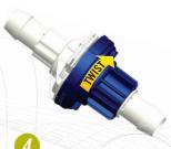
Twist the blue lock ring clockwise until the final audible "CPC Click" is heard (90° from the initial starting point). Alignment of the long blue lock ring rib indicator with the white body's rib indicator confirms initial rotation is complete.
