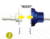
Align male and female connectors using the START alignment feature of the blue lock ring with the rib indicator of the white body. Insert the two halves together.
